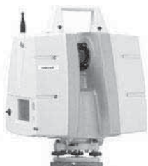
Sl. 6. Terestrički laserski skener (Terrestrial laser scanner)
